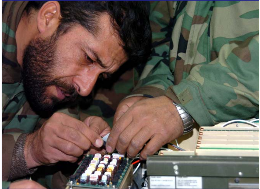
Said Forouk, Ministry of Defense Communication Officer, takes a close look at a radio component to determine pin alignment of a connection.
